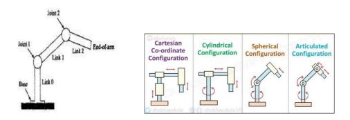
Fig: Robot Anatomy and configurations
